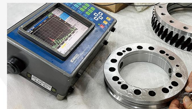
RACEWAY QUENCHING DEPTH DETECTION
